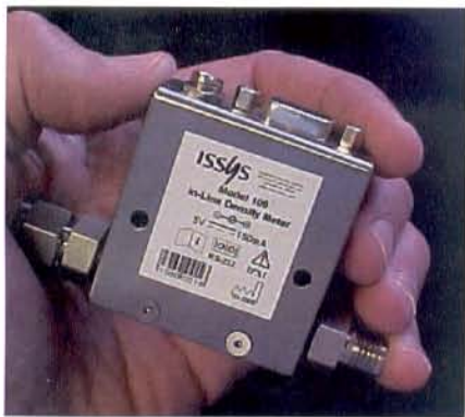
Figure 1. A MEMS-based chemical concentration/density sensor
