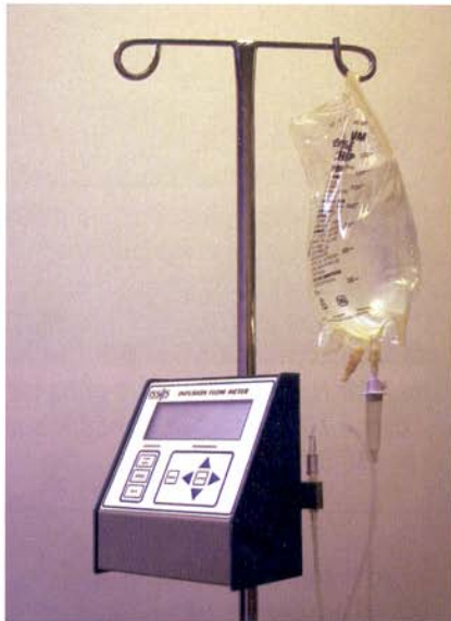
Figure 4. Drug flow monitor using micro Coriolis mass flow sensor
