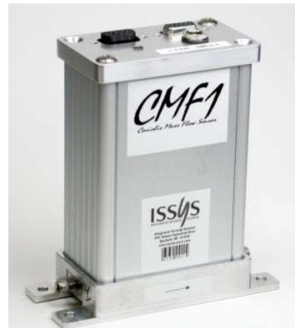
Fig. 4. Final packaged MEMS-based, industrial Coriolis mass flow sensor.
