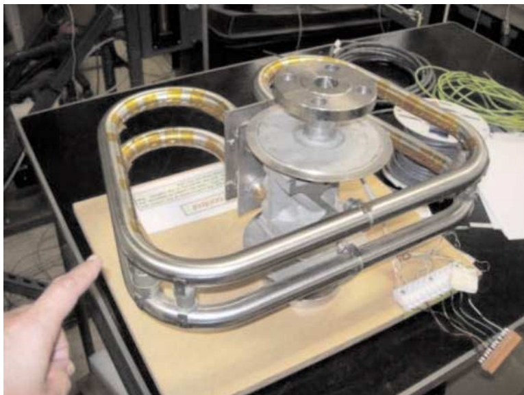
FIG. 8—Example of a stainless steel tube Coriolis mass flow/density metres.
