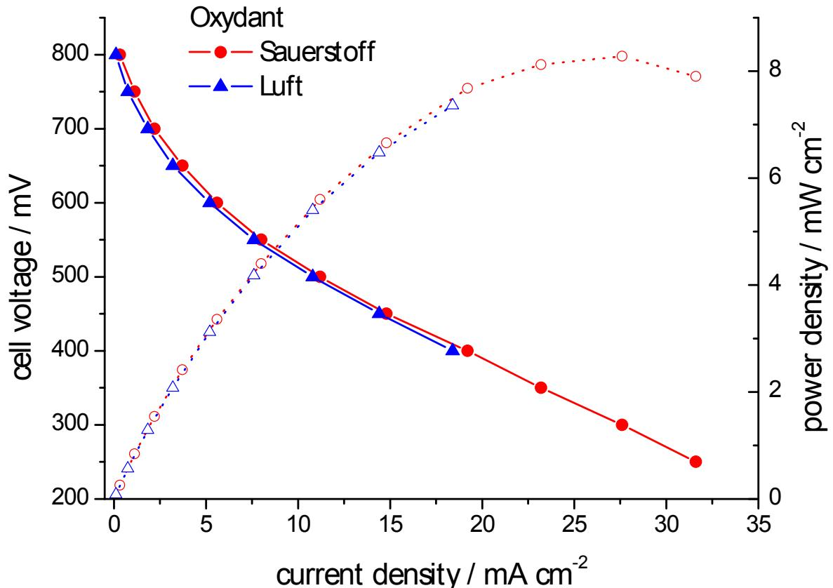
*Performance of a DEFC single cell with Fraunhofer IGB sPEEK composite membrane and Fraunhofer ICT electrodes
