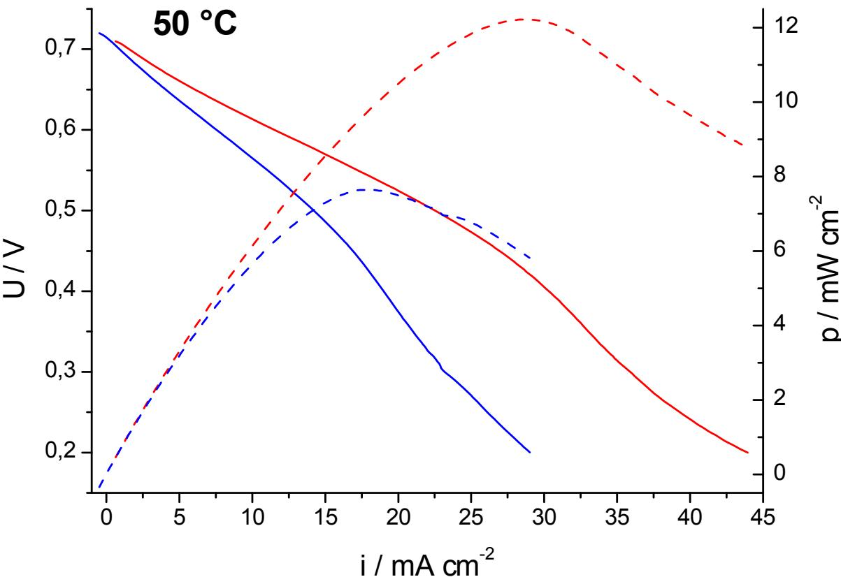
I-V and I-P curves of DEFC single cells with a PtSn/C (blue) and a PtSn/C + PtRu/C anode measured at 50 °C, with 1M ethanol and air as the oxidant.
