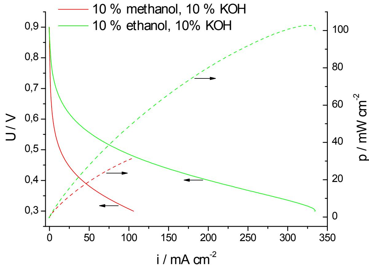
I-V (straight) and I-P (dashed) curves of an AEM based DAFC using Acta S.p.A. Hypermec GDEs and a Fumatech Fumasep FAA membrane operated with methanol or ethanol, 50°C, air.
