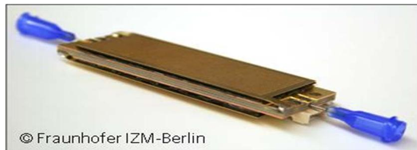
4-cell-stack with two bi-cells
