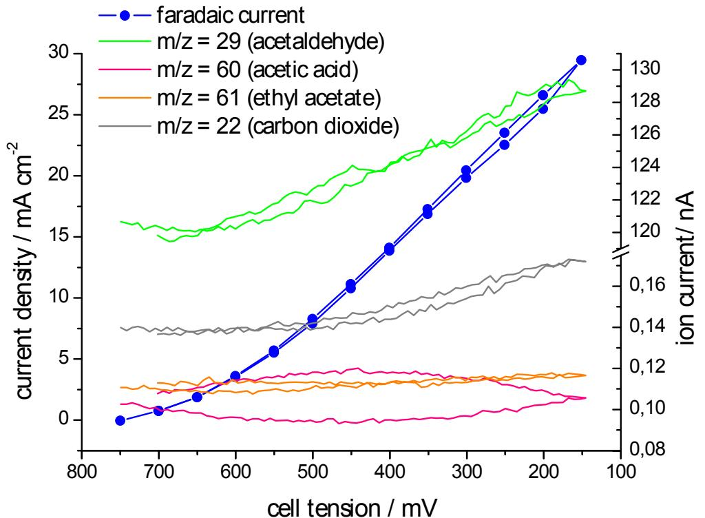
Single cell tests with online MS analytics of the anolyte for single cells with a PtSn/C anode with  $3.4 \text{ mg/cm}^2$  (left) and PtSn/C + PtRu/C anode with a total of  $1.8 \text{ mg/cm}^2$  (right); measured at  $40^\circ\text{C}$  with 1M ethanol and oxygen as the oxidant.
