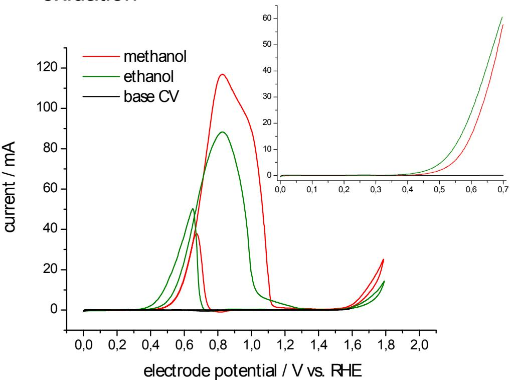
CV of the methanol and ethanol oxidation in 0.5 M KOH at platinum at ambient temperature
