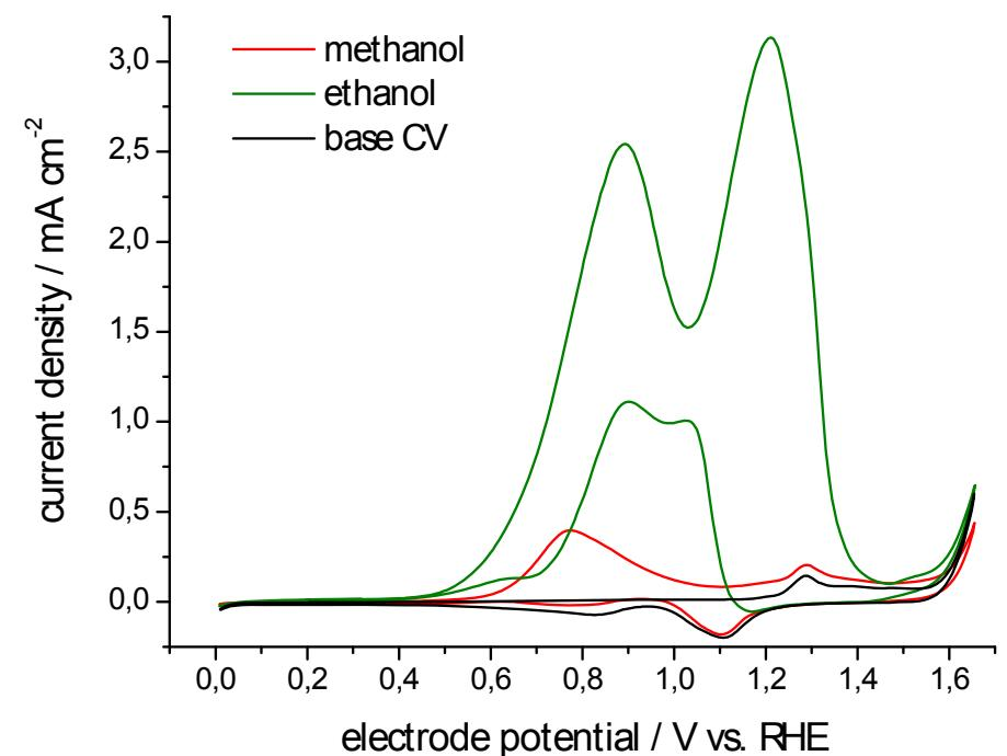
CV of the methanol and ethanol oxidation in 0.5 M KOH at gold at ambient temperature
