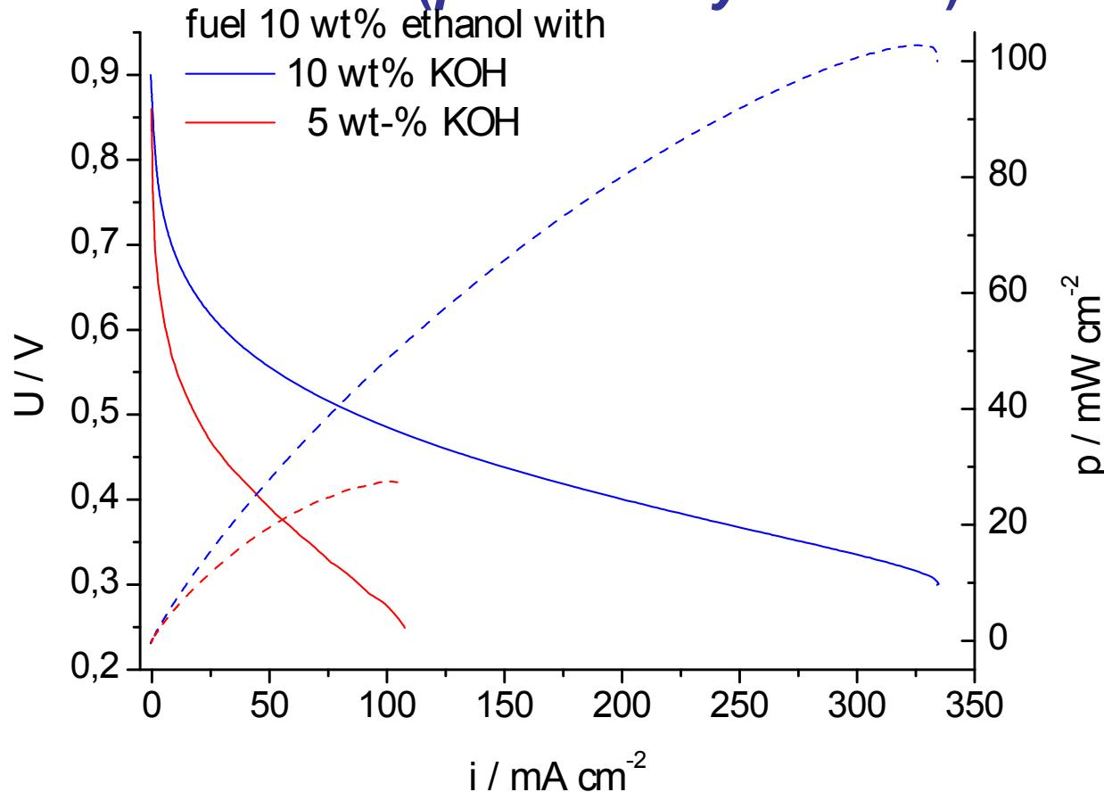
I-V (straight) and I-P (dashed) curves of an AEM based DEFC using Acta S.p.A. Hypermec GDEs and a Fumatech Fumasep FAA membrane fuelled with ethanol in 10% and 5% KOH, 50°C, air.
