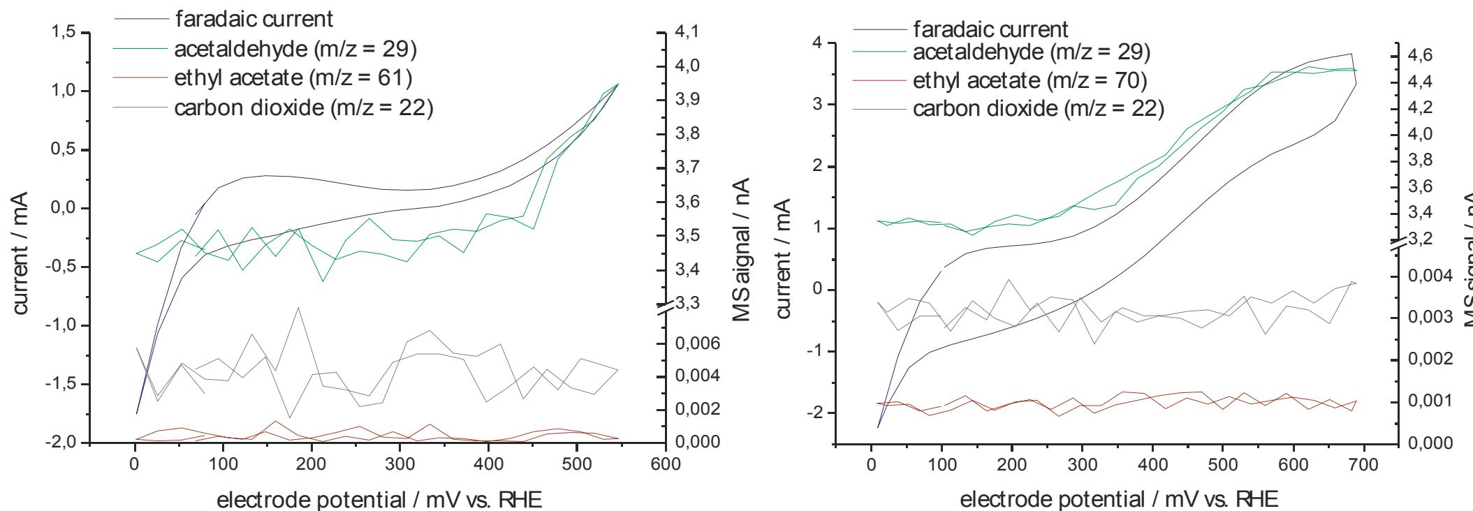
MSCVs of the ethanol oxidation at a Pt (left) and a PtSn electrode (right), recorded in a 1M ethanol, 0.5M sulphuric acid solution at ambient temperature, sweep rate 20 mV/s.
