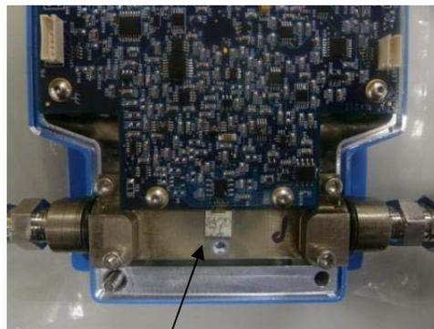
**Fig. 7.** MEMS integration into the industrial inline density meter.
