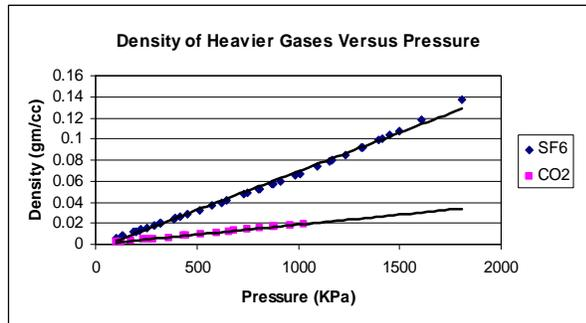
Fig. 4. The density of sulfur hexafluoride and carbon dioxide versus pressure.
