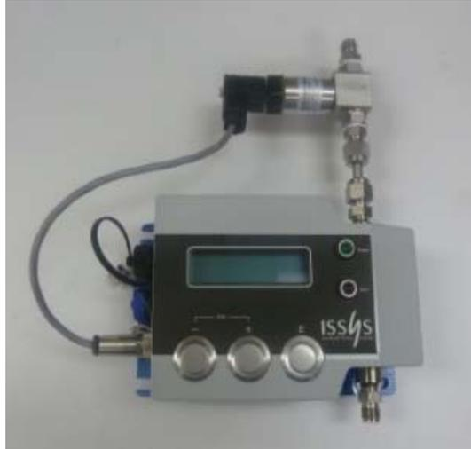
Fig. 1. The density meter (bottom) and pressure sensor (top).
