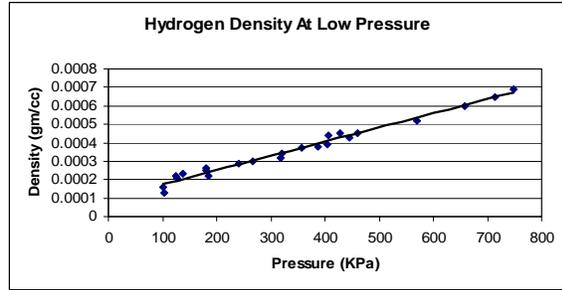
Fig. 3. The variation of hydrogen density with pressure in the range of 101 to 750 KPa.
