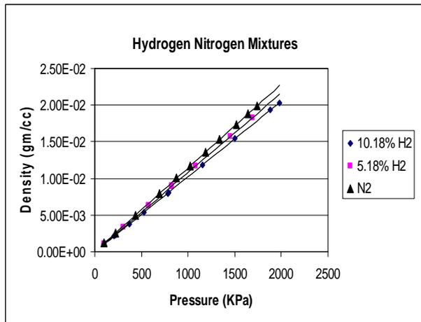
Fig. 5. The variation in gas mixture density with pressure for different nitrogen-hydrogen mixtures.
