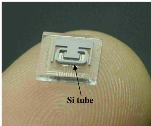
**Fig. 6.** The MEMS chip and resonating microtube.
