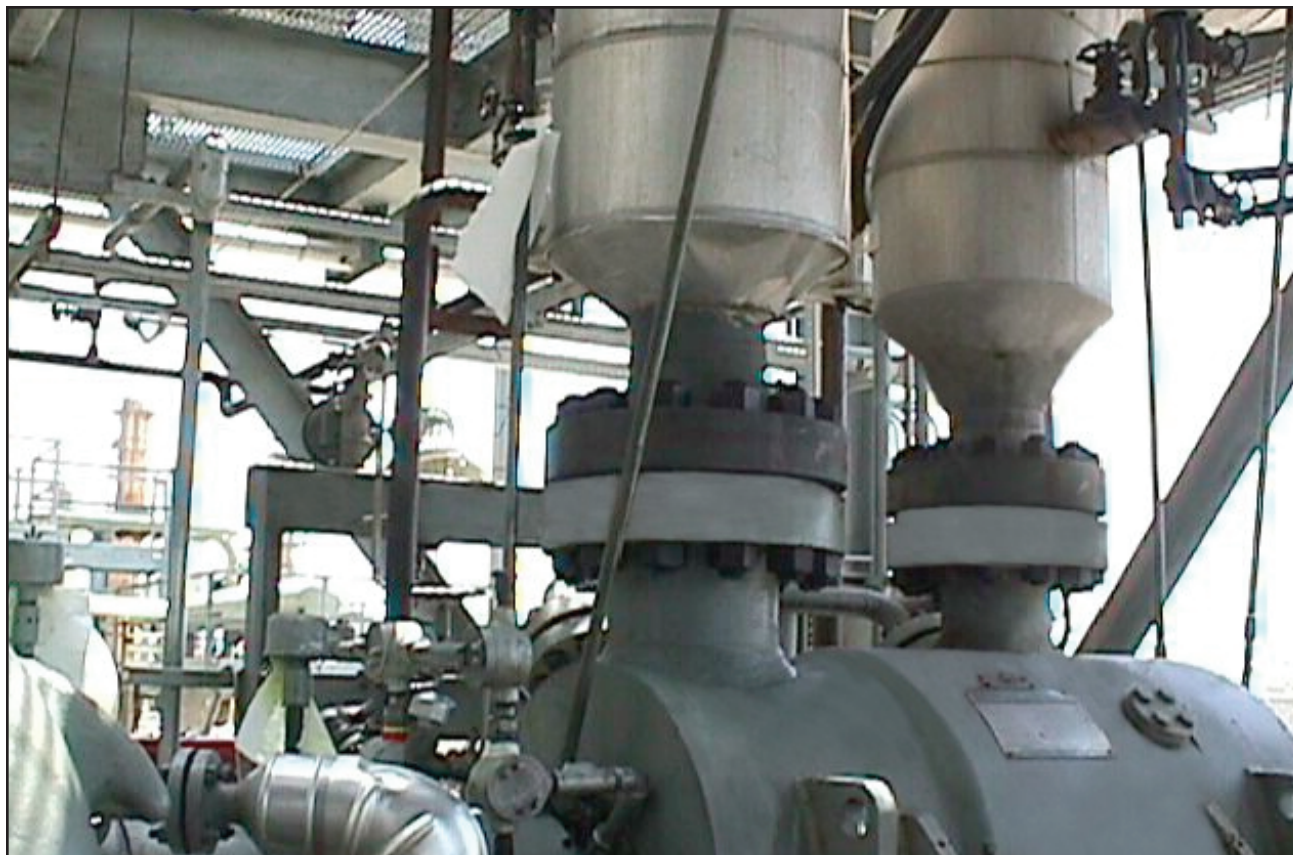
■ Elliott 15 MB hydrogen recycle compressor at the Valero refinery in Ardmore, Oklahoma, U.S.A. Performance analysis found that cleaning the compressor would bring the unit back to normal operating conditions and a rerate was not necessary. Plans are to install online performance monitoring software to confirm current performance and to aid in scheduling compressor maintenance.
