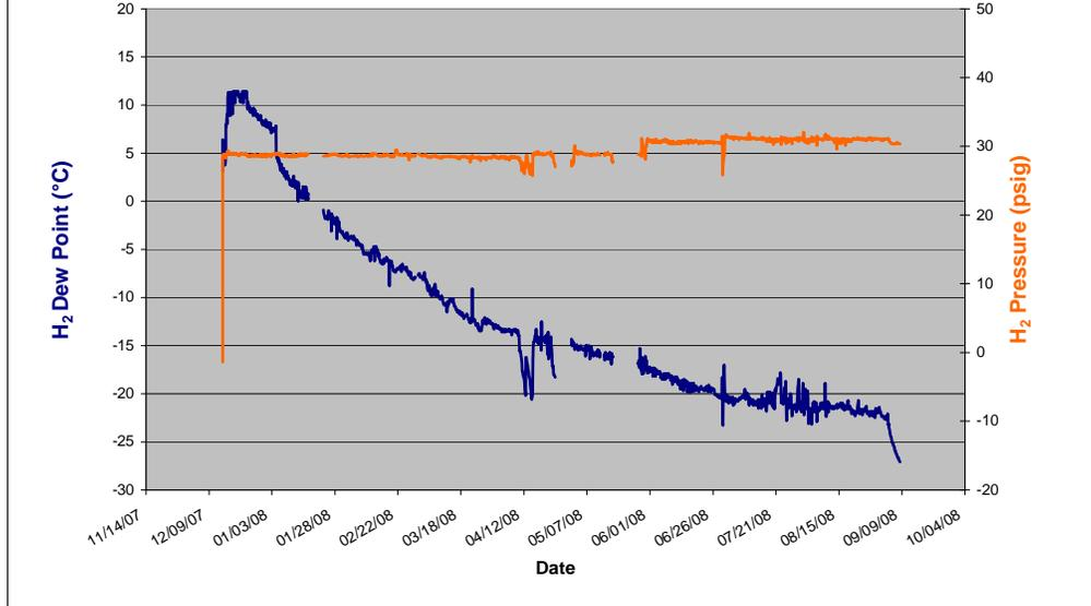
Either a dryer in the recycle loop, or an optimized scavenge system can control hydrogen dewpoint. This chart illustrates the performance of a StableFlow hydrogen control system driving dewpoint to manufacturer compliant levels without a dryer. Note the pressure stability – the benefit of optimized constant scavenge.
