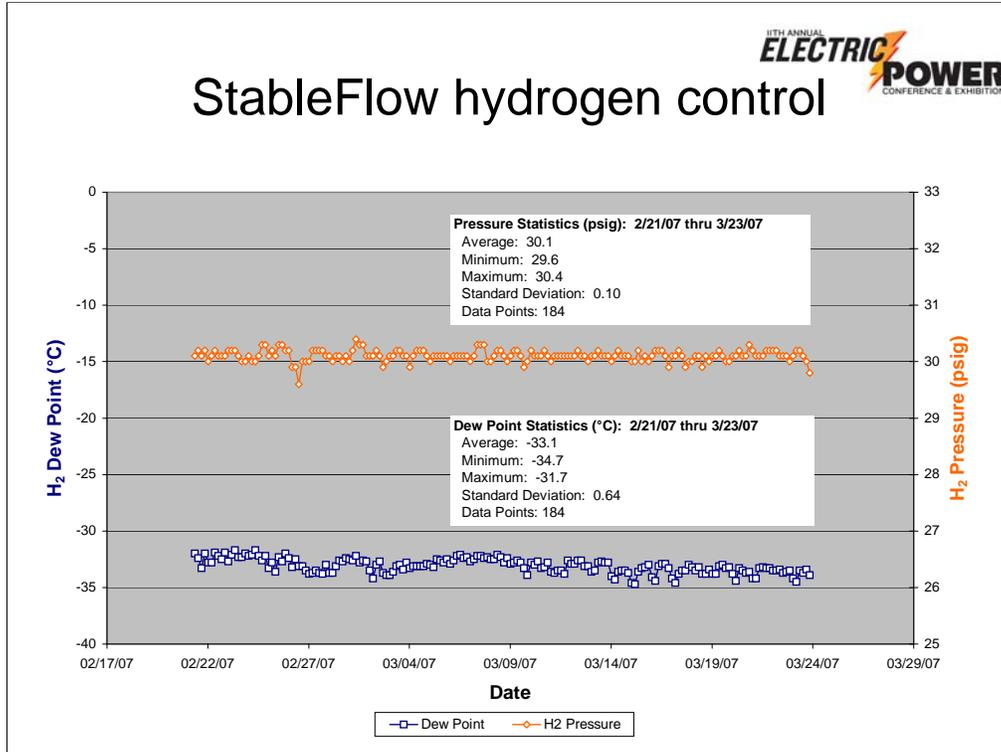
StableFlow hydrogen control system – stable, compliant hydrogen specifications translates into maximum generator performance and lifetime
