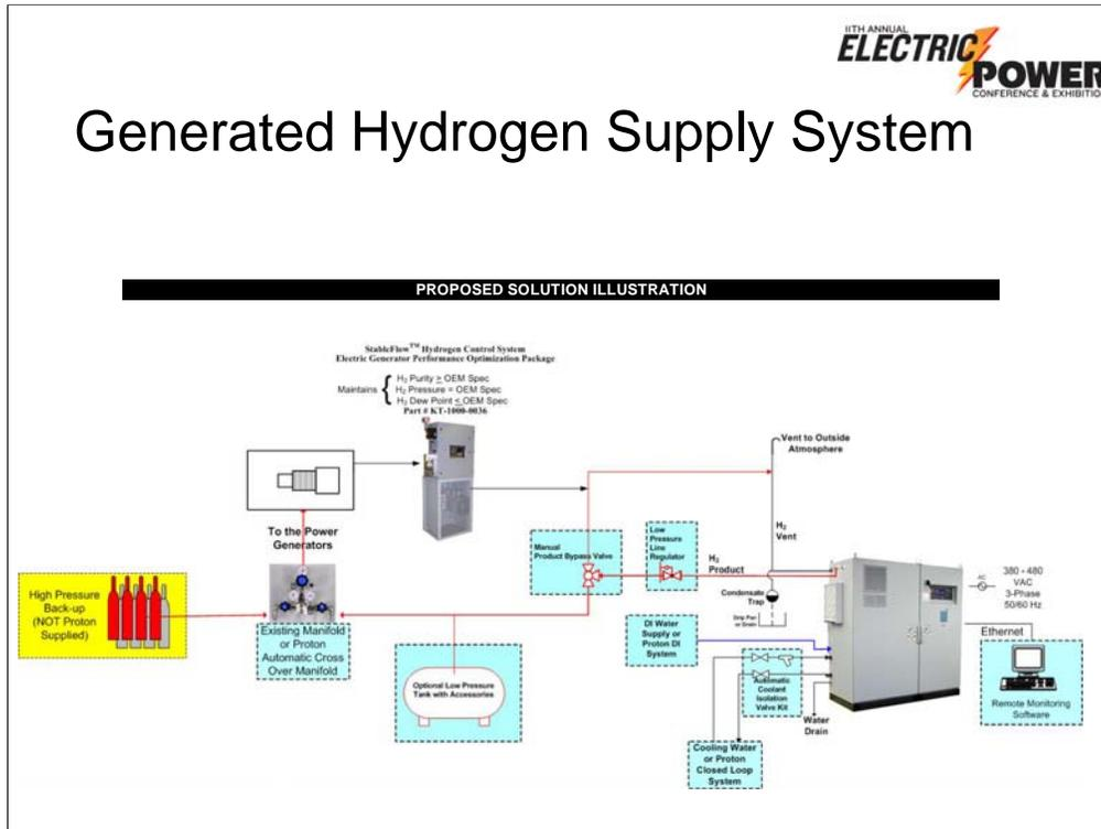
Generated hydrogen doesn't eliminate the need to store hydrogen for regas – but it does dramatically reduce the size of storage required, and offers the opportunity to make your own regas hydrogen, eliminating deliveries entirely.
