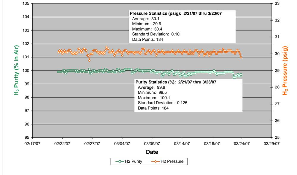
StableFlow hydrogen control system – stable, compliant hydrogen specifications translates into maximum generator performance and lifetime
