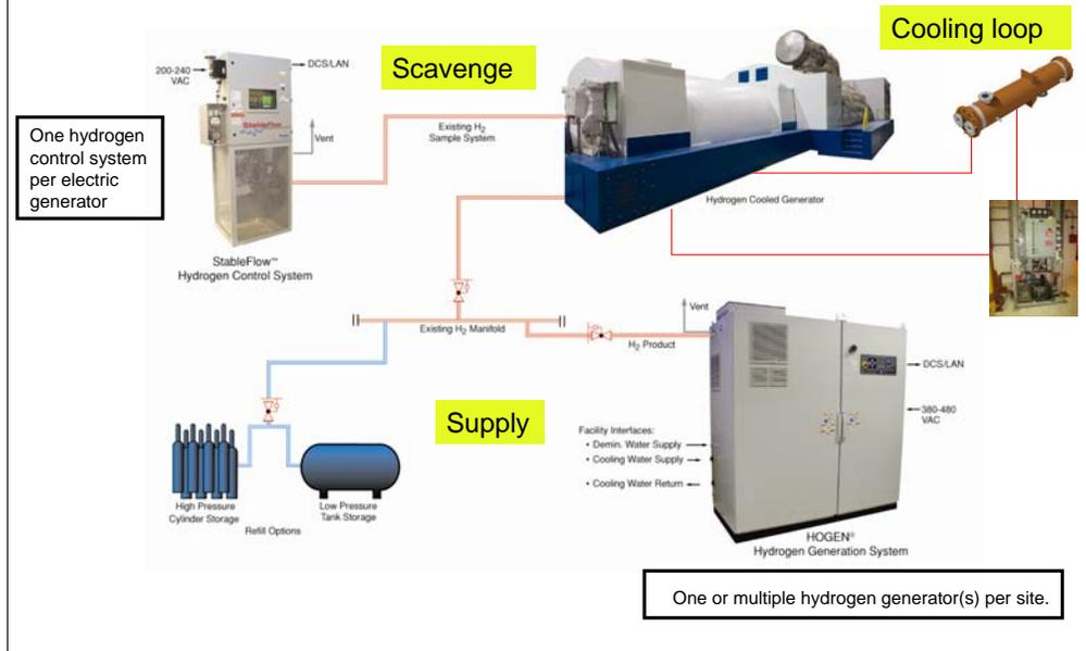
This is a standard hydrogen-cooled generator equipment layout. There are basically three hydrogen “systems” – the hydrogen supply side of the generator, the hydrogen recirculating cooling loop, and the hydrogen scavenge portion of the system. Hydrogen safety and quality can be affected by the choice, capabilities, and operation of the technologies in each of the systems.
