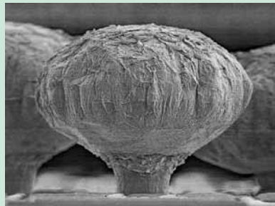
(a) first-reflowed at 400°C for 8 min. in N 2 with 100 ppm O 2
