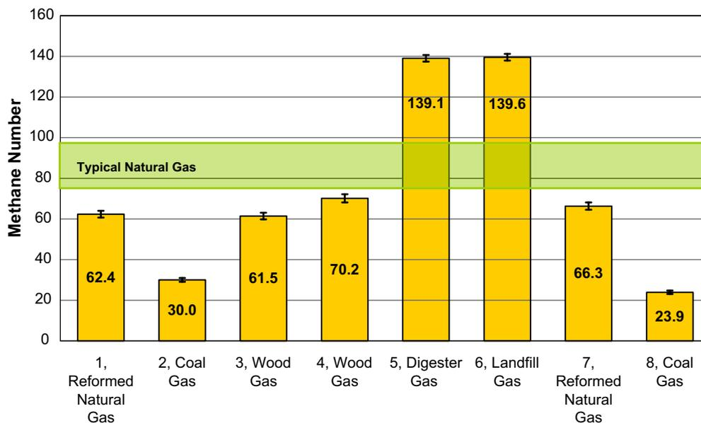
Fig. 3. Methane number results for simulated fuels, for run 2.
