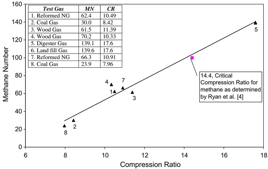
Fig. 4. Test gas compression ratio vs. measured methane number.
