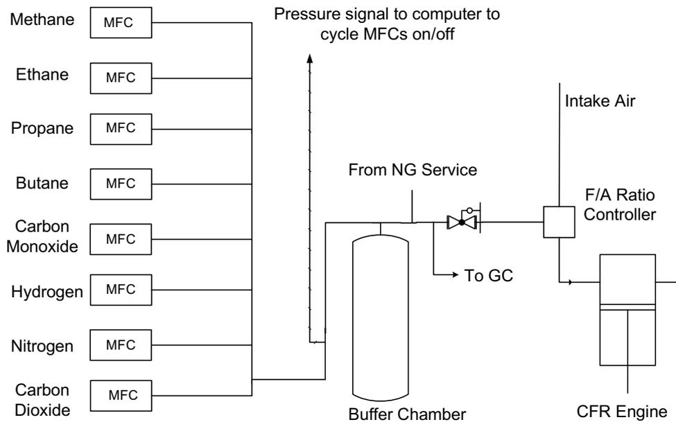
Fig. 1. Schematic of gas blending system.
