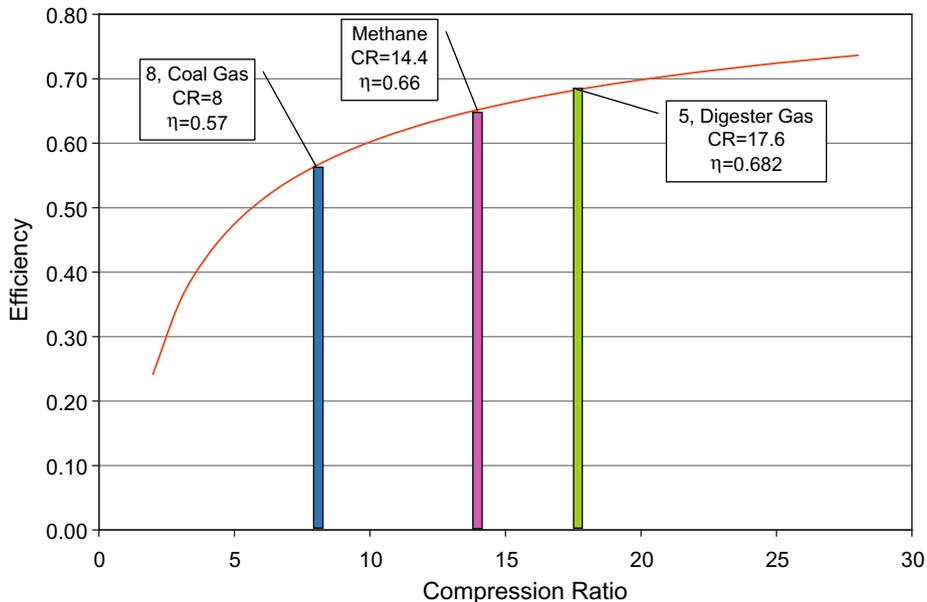
Fig. 5. Theoretical efficiency of simulated alternative gaseous fuels.
