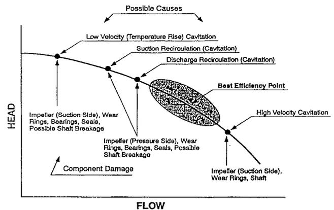
Figure 2. Centrifugal Pump Component Damage and Causes.
