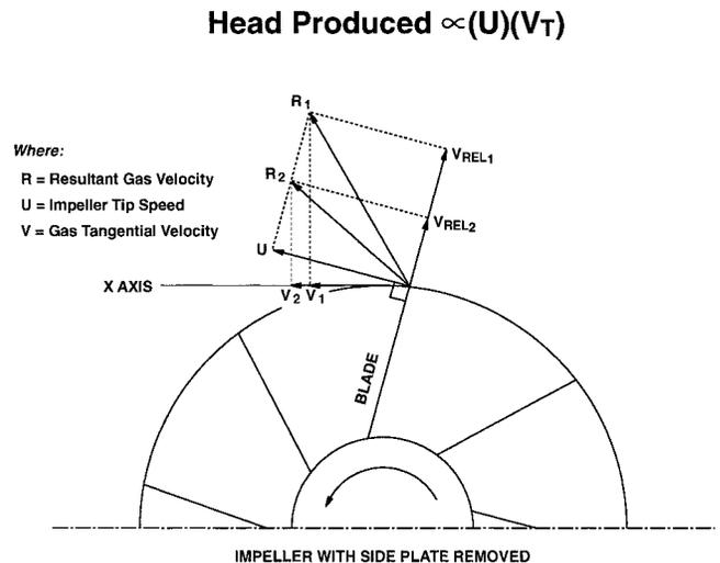
Figure 6. Simplified Turbocompressor Discharge Triangle for Two Flow Cases.
