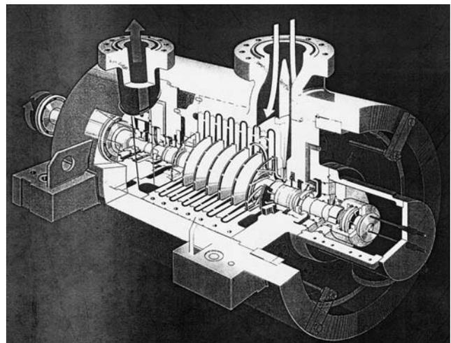
Figure 3. Barrel Compressor Assembly Drawing. (Courtesy Siemens/Demag Delaval)
