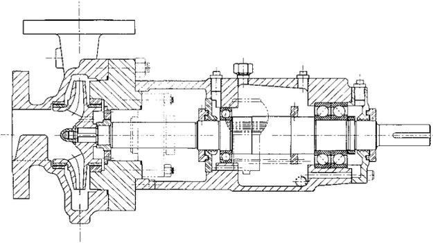
Figure 1. Diagram of Centrifugal Pump.
